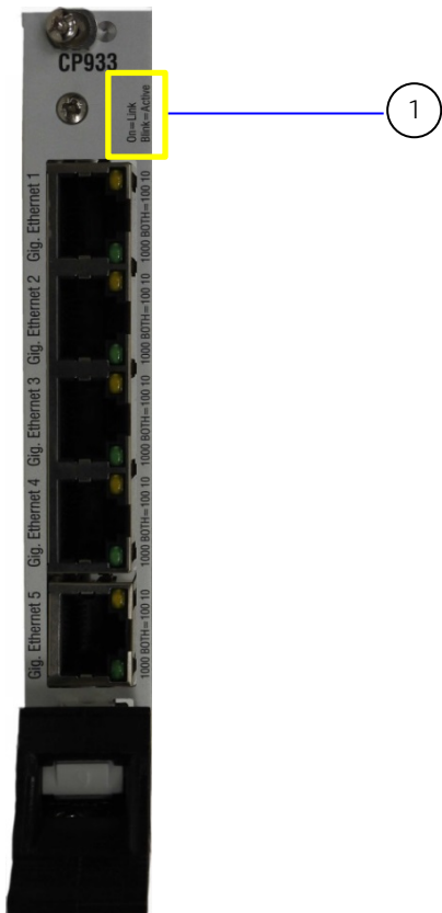
Figure 5: Front Panel LED Activity
